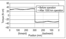
Torque: Comparison of torque values of low particle-generating grease types
