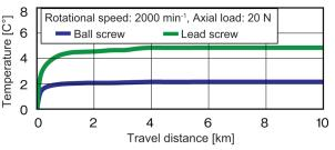
Outstanding temperature characteristics: Low heat generation ability that can only be realized by ball screws
