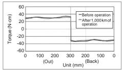
Delivers stable torque characteristics even during oscillating operation.
